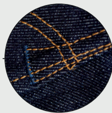
The fly is reinforced by an indigo dyed bartack to prevent ripping
